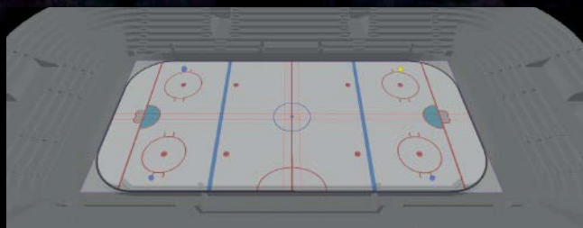
^ Playing surface alignment projection system before alignment
